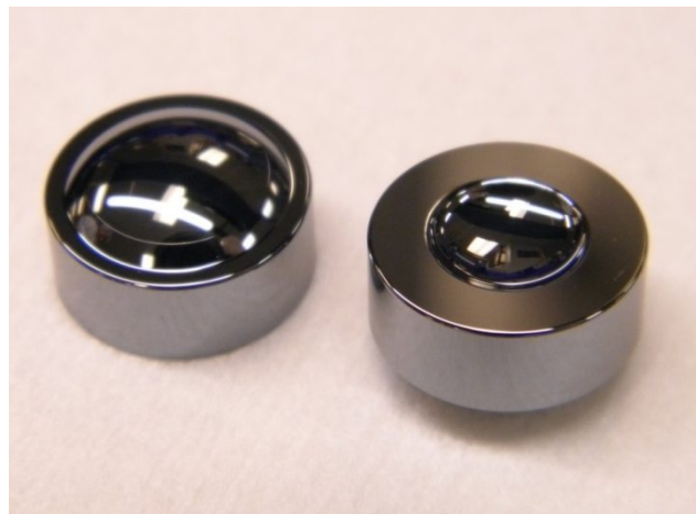
Figure 8 - Image of Successfully Molded As_{40}Se_{60} Lenses
