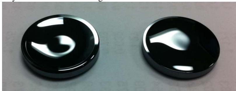
Figure 5: Both Surfaces of Aspheric bi-Gullwing Lens
