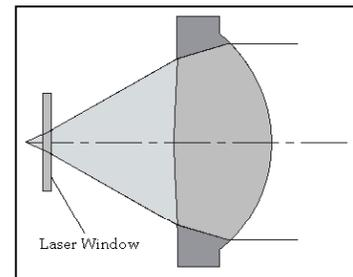
**Figure 3:** Example of an asphere with a laser window.
