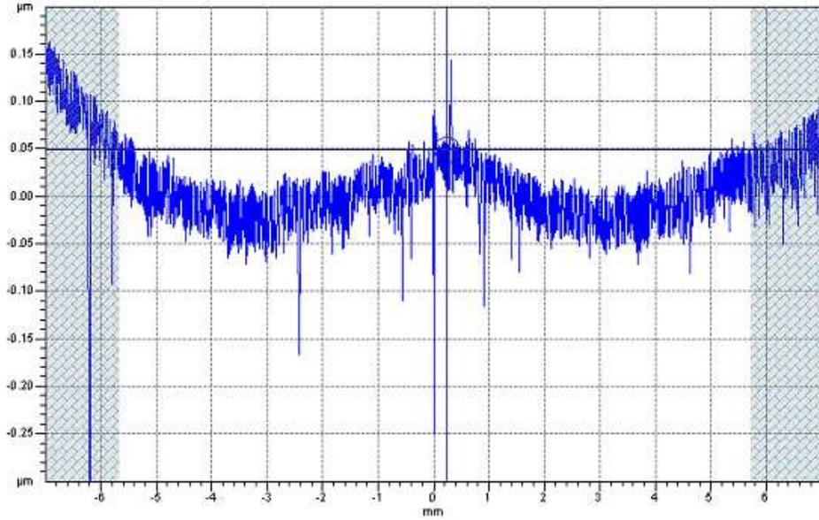
Figure 7: Aspheric surface profile error (with adjusted radius).
