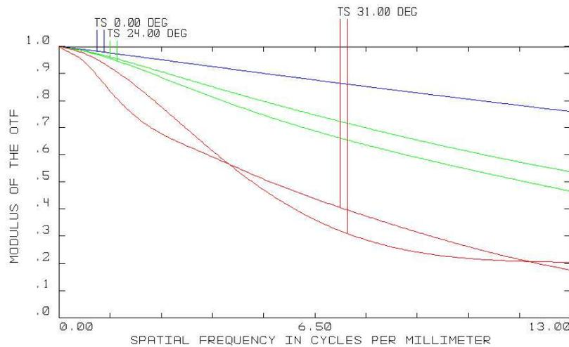
Figure 3: Polychromatic MTF plots on-axis, at  $24^\circ$ , and at  $31^\circ$ .
