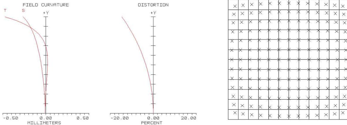
Figure 4: Left: field curvature and distortion plots (vertical axis is the field angle 0 to  $31^\circ$ ). Right: grid distortion.
