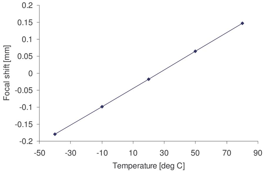
Figure 8: Focal shift versus temperature.
