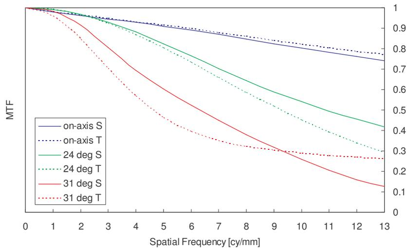
Figure 9: Measured MTF on-axis, at 24°, and at 31° (solid-sagittal, dashed-tangential).
