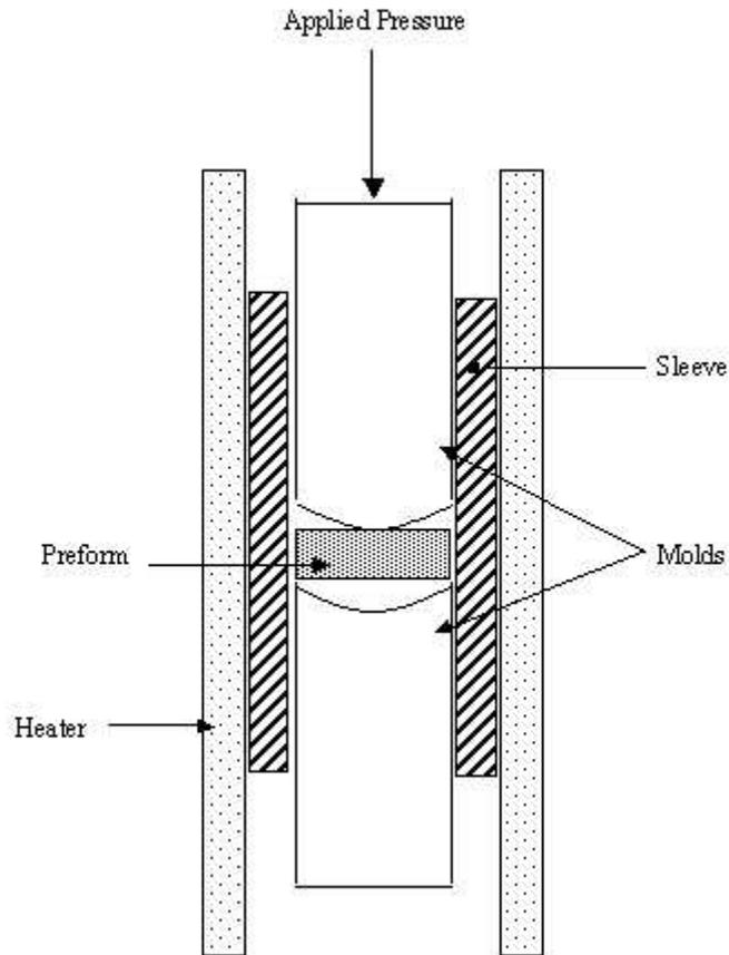
Figure 1: Schematic of chalcogenide glass pressing apparatus.
