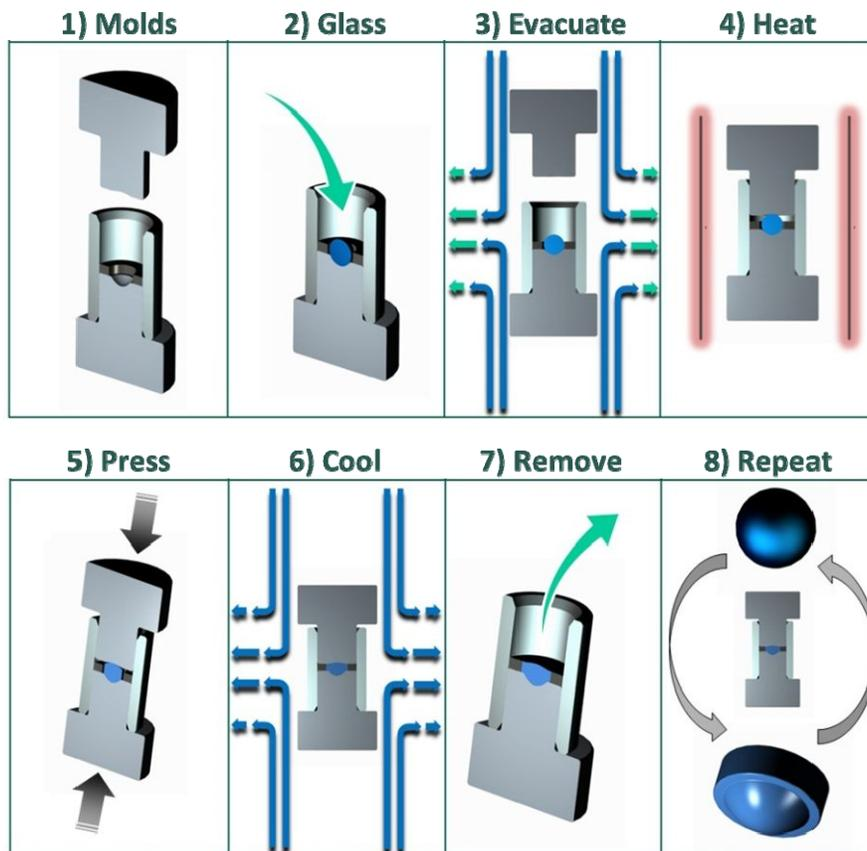
**Figure 1 - Precision Glass Molding Sequence**
