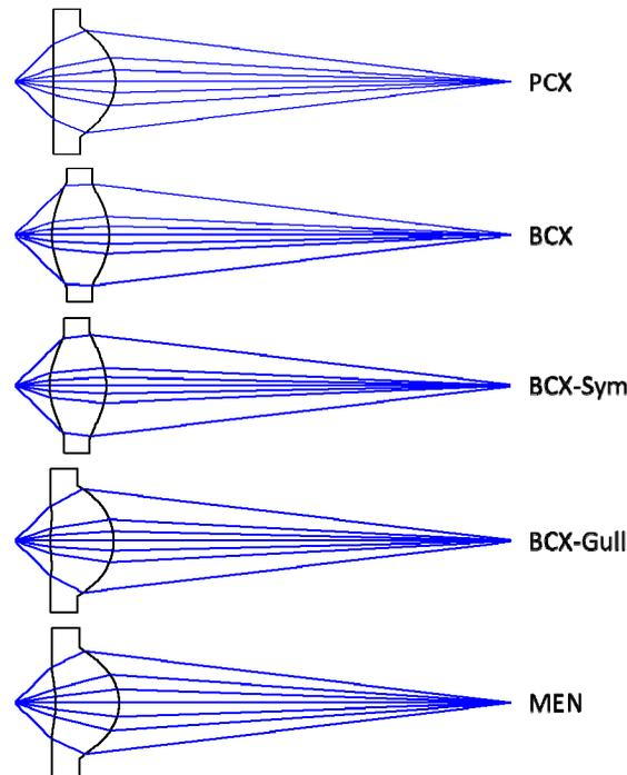
**Figure 5** - *Adjusted lens forms for designs optimized to meet manufacturing design rules*
