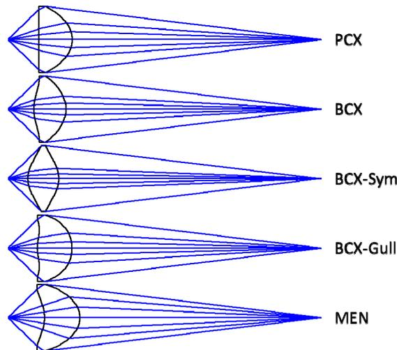
**Figure 4** - Singlet lens forms, unconstrained by manufacturing design rules
