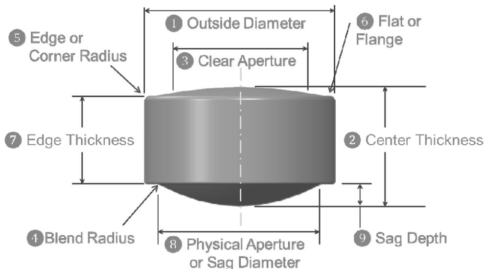
**Figure 2** – Description of a well-designed bi-convex precision glass molded aspheric lens
