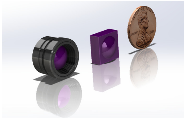
Figure 5 Equivalent Design – Left: Traditional / Right: Wafer Level
