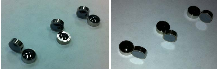
Figure 5: BD2 glass molded inside a MIP ring
