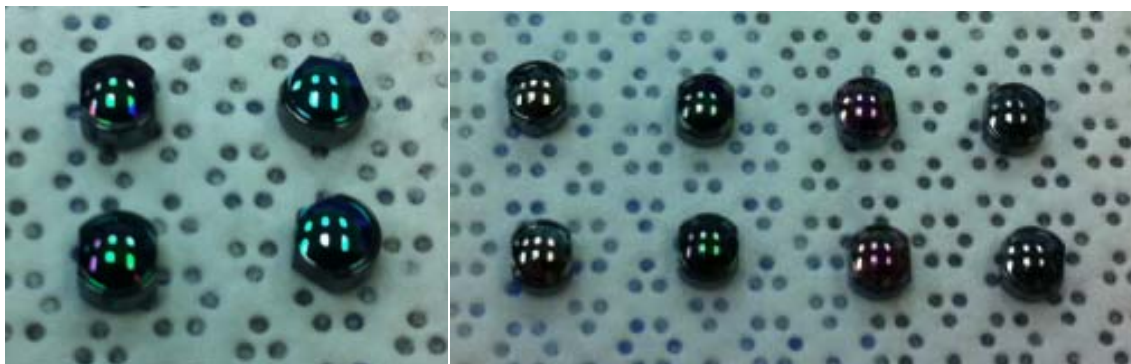
Figure 2: Different geometrical and AR coatings of diced lenses
