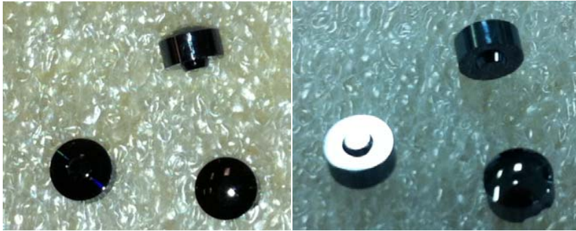
Figure 7: Molded BD2 glass lenses with stepped feature
